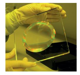
Structured CGH on a 6-inch mask blank (152 mm x 152 mm x 6.35 mm).
